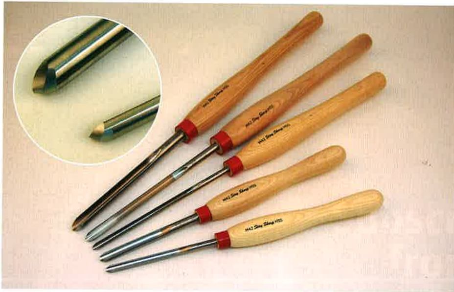
The tools received for testing and close-up of a bowl gouge and spindle gouge tip
