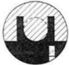
**2a** With a suitable parting tool, cut to a depth equal to, or slightly deeper than, ring diameter.
