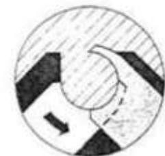
**4a** Locate the nose of the RH side of the tool very lightly against the bead and rotate the cutter 90 degrees anti-clockwise. Avoid pushing the tool forward into the work as this will reduce the diameter already cut with the Bead Forming Tool.
